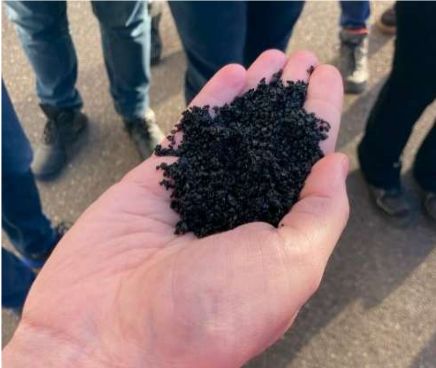
Granular Activated Carbon from BODAC NieuWater UPW Emmen
